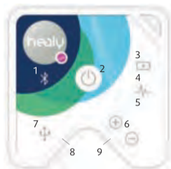
Figure 2.4.1.1: Healy top view: Pos. 1 Icon and LED for Bluetooth Connection; Pos. 2 On-Off Button; Pos. 3 Battery icon, Pos. 4 LED for generator action (if stimulator output is active, then the LED is blinking) and battery indicator; Pos. 5 Generator icon; Pos. 6 Icons for the positive and negative electrode plugs; Pos. 7 USB-Connector icon; Pos. 8 Socket for power supply
